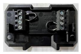
To run the fan all the time, place the jumper wire between FAN and 24VAC. The fan will
