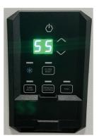
B. "tc" on the display indicating terminal control. Press the "TERMINAL CONTROL" button so the light is NOT illuminated, and humidity set point is displayed as above.
