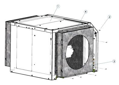
ITEM 1: Quest 225 Dehumidifier (not provided) ITEM 2: #10-24 Panhead Torx Screws (6) ITEM 3: Duct Plenum Face (1) ITEM 4: Exhaust Duct Plenum (1) ITEM 5: 14'' Dia. Duct Collar (not provided)\* ITEM 6: 1/8'' Drill Bit (not provided)\*
