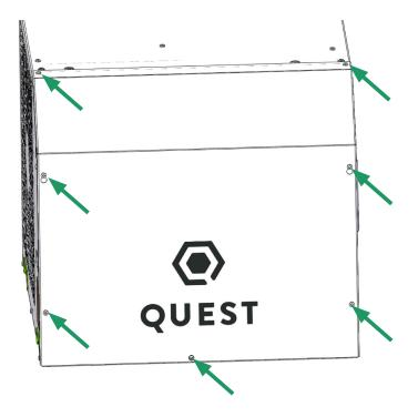
Remove 7 screws on access panel using T25 Torx driver, remove panel.
