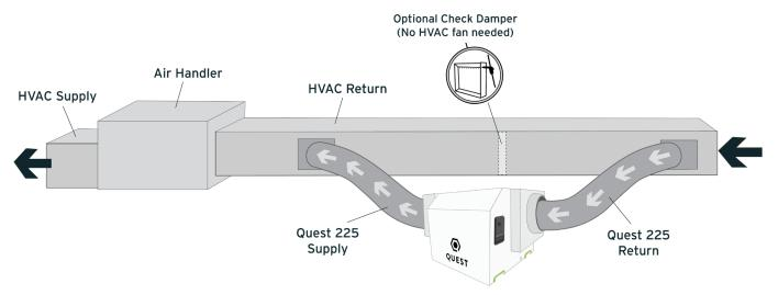
NOTE: If Check Damper is not in place, the HVAC fan must ON when the dehumidifier is in operation.
