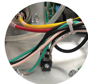
HIGH VOLTAGE POWER BLOCK FOR CORDED OR HARDWIRED INSTALLATION
