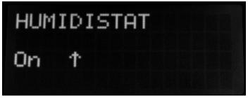
Press the Next button to advance to the next screen. If Humidistat mode is enabled, then proceed to Humidistat Set point. Else, proceed to Humidity Units.
