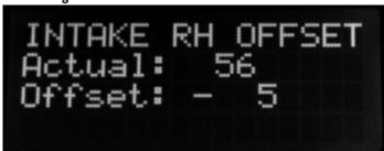
The Intake RH Offset allows you to calibrate the CDG 74 to match your favorite meter.
