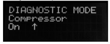
Press the Set button to toggle the Compressor On/Off.
