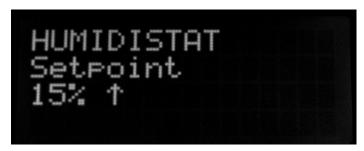
Press the Set button to adjust the set point RH% in 5% increments ranging from 20% RH to 80% RH and then looping back to 20% RH.
