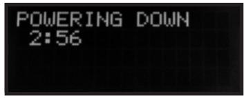
The default shut-down time is three minutes plus 20 seconds for a final purge. The shutdown time can be changed be scrolling through the menu to this screen.
