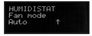
Press the Set button to toggle the Humidistat Fan mode from Always On to Auto.
