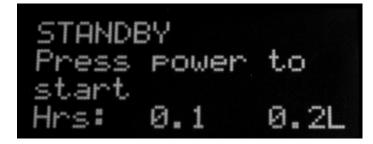
When plugged in, the display will communicate to the user that the machine is in Standby mode and ready to be powered on. In Standby Mode, the display will also show the current job and life hours on the fourth line.
