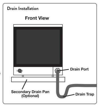
Use care to keep the hose as flat to the floor as possible after your trap is in place. Be sure the hose is not kinked or otherwise restricted so water can pass through the hose freely. Improper installation of the drain hose may result in water leakage.
