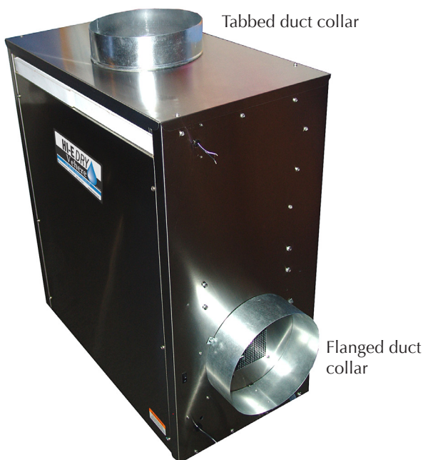
Figure 8: Tabbed duct collar is installed around the exhaust outlet. The flanged duct collar is installed around the intake opening.
