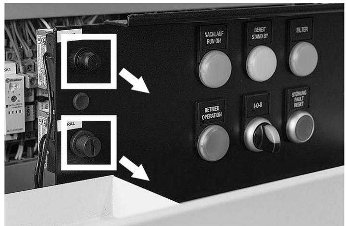
2. Press the corresponding reset button and reattach the cover.
