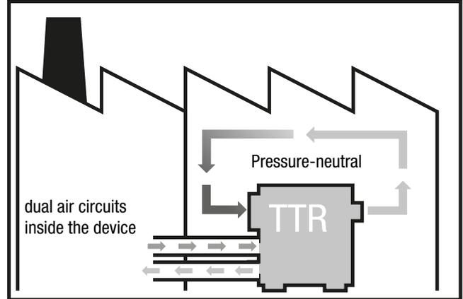
**Circulating air for drying outdoor installation**
