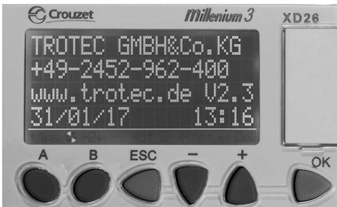
1. Within the screen you can move up and down using the buttons **+** and **-**.
