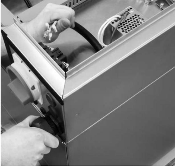
3. Guide the mains cable through the cable gland at the device and connect it to the power supply terminals. To connect the device please observe the wiring diagram in the technical annex. The phase sequence can be chosen freely.
