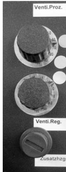
The upper "Venti.Proz." potentiometer serves to define the target value for the process/dry air volume in m<sup>3</sup>/h. The topmost point roughly marks the regulated nominal air volume and the point in the middle marks the nominal air volume in emergency operation. The points indicate the rough settings for emergency operation (failure of Flowmatic S).
