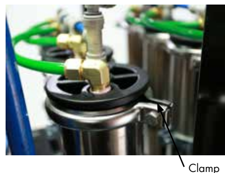
FIGURE 56-1: ANDEN REVERSE OSMOSIS MEMBRANES
