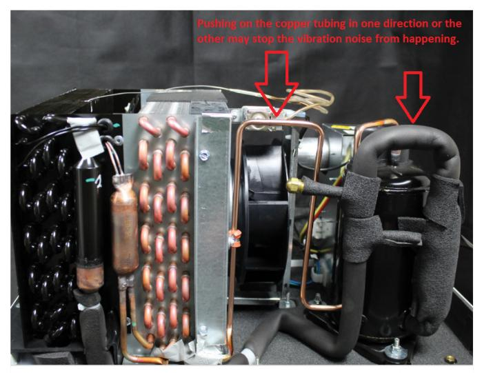
Tightening or loosening the compressor mounting bolts may stop any vibration noise from cabinet.
