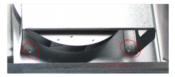
7. Remove the fan bracket and impeller fan assembly from the unit. The wiring for the fan has a rubber sleeve on it that runs through the metal fan shroud. This will pull out of the metal shroud. The rubber sleeve is separated to remove from the wire. Reuse this on the new impeller fan assembly.
