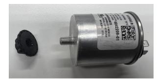
10. Connect wires to capacitor. Blacks go together. Brown on the opposite side of terminals.
