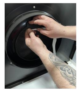
Reinstall exhaust and access panel and retest unit.
