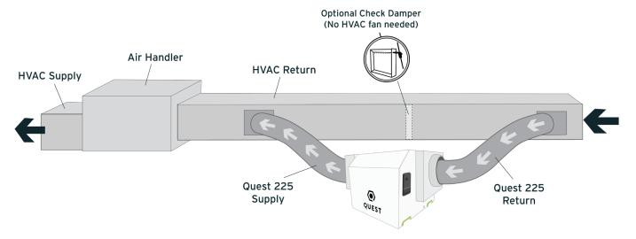
NOTE: If Check Damper is not in place, the HVAC fan must ON when the dehumidifier is in operation.
