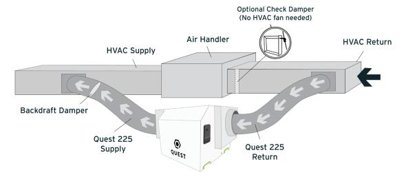
Check damper should be in place between the Return and Supply connections of the dehumidifier.
