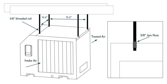
Parts Needed: 4 pieces 3/8" threaded rod (not included) 4 - 3/8" threaded jam nuts (not included)
