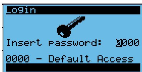
2. Press Enter four times to access the menu. Then, press Up/Down keys until Settings is highlighted.
