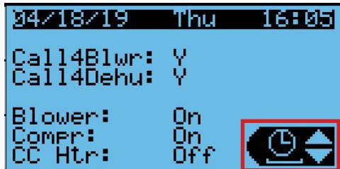
2. Press Enter to display the operating hours for the entire unit (compressor or fan), for the blower, and for the compressor.
